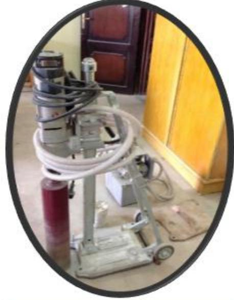
Concrete core sampler
